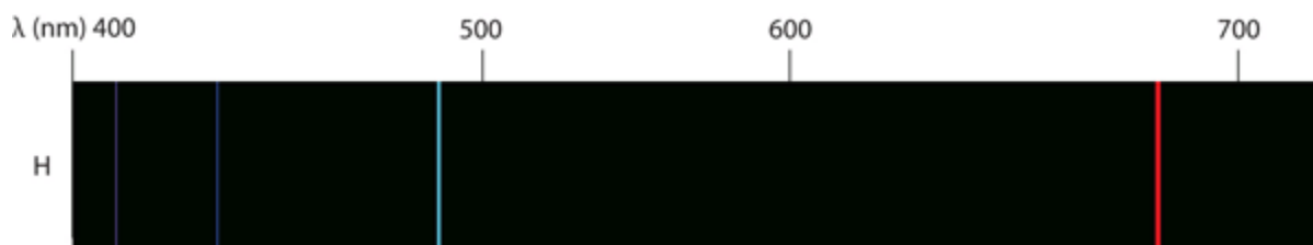
Figure 8.04 “Hydrogen Spectrum.” The spectrum of hydrogen was particularly simple and could be predicted by a simple mathematical expression.
