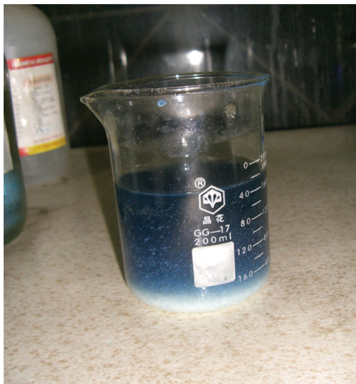
Figure 4.2 “Double-Replacement Reactions.” Some double-replacement reactions are obvious because you can see a solid precipitate coming out of the solution.
