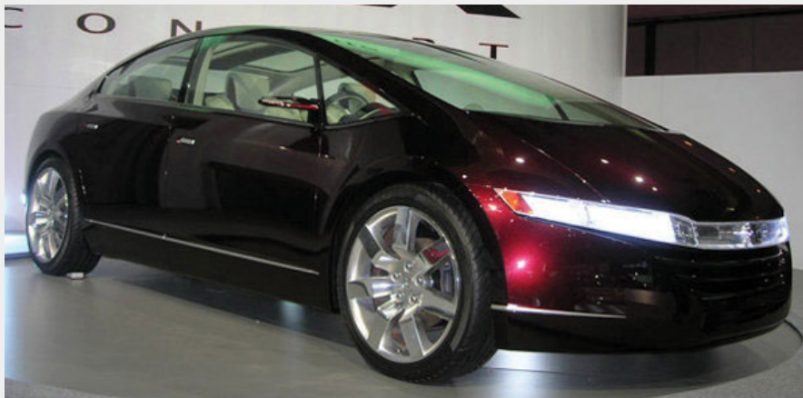
The 2008 Honda FCX was the first production car to use a fuel cell as a power source. Nonetheless, the car is in very limited service because of its need for relatively large quantities of elemental hydrogen as fuel.
