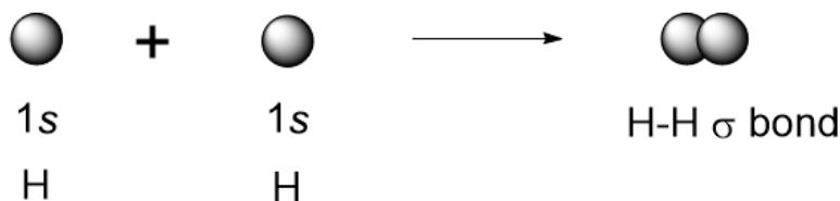
Figure 9.6. A diagram showing the overlap of s orbitals of two hydrogen atoms to form H_2 .
