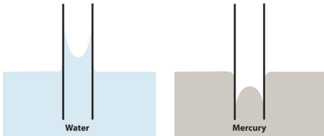
Figure 10.10 “Capillary Action.” (a) Capillary rise is seen when adhesion is strong, such as with water in a thin glass tube. (b) Capillary depression is seen when cohesive forces are stronger than adhesive forces, such as with mercury and thin glass tubes.
