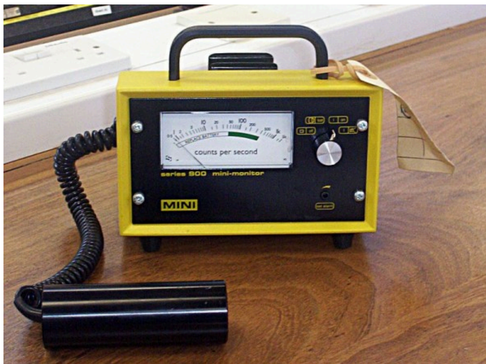
Figure 15.1 “Detecting Radioactivity.” A Geiger counter is a common instrument used to detect radioactivity.
