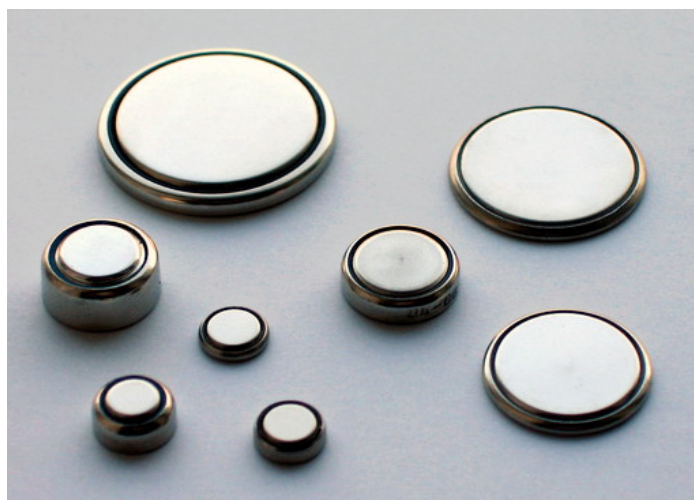
Figure 14.3 “Button Batteries.” Button batteries like those seen here can be used for a variety of portable electronics, from watches and hearing aids to handheld gaming devices.
