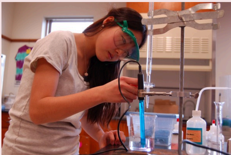
When a student performs a titration, a measured amount of one solution is added to another reactant.
